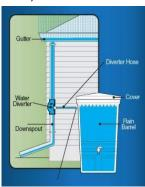
base you will be measuring a level line over to your down spout, then depending upon the diverter type, you may be installing the diverter slightly above the level line to ensure that water diverts to the rain barrel. Overflow will continue down your existing down spout.
