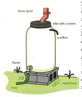
Solutions website has a good installation video. Essentially, after establishing your base, you will remove elbow from lower part of down spout, determine where to cut your downspout above your barrel, and re-attach the elbow. A flexible piece of gutter can ease this process. Be sure that the overflow pipe directs water away from your house.
